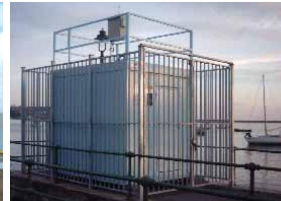
The air quality control stations network of the Bilbao Port Authority consists of an Automatic Weather Station and three fixed measuring cabins.
